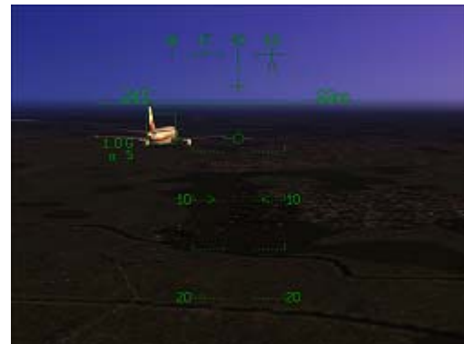
At less than 1 NM, the distance information disappears. The target is now visible.
