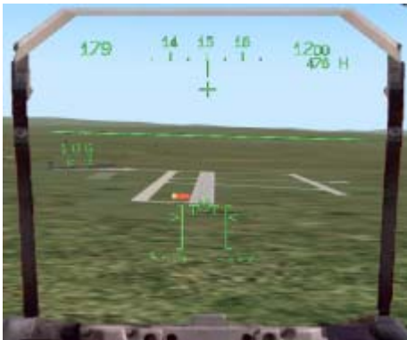
The situation is good but the speed vector is almost out of the incidence range.
