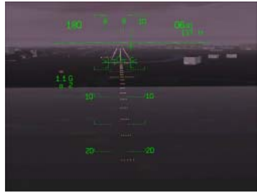
Close to land, the aircraft situation is perfect: airspeed is good, the flight path vector is aligned with the runway and still in the incidence range, the speed is constant and the gear is OK.
