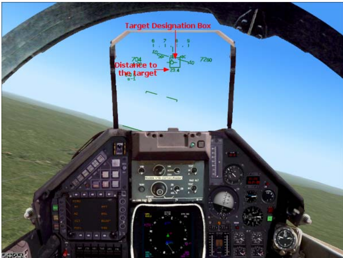
The target is at 23.4 NM, beyond visual range. The flight path vector is aligned with the target designation box to fly directly to the target.
