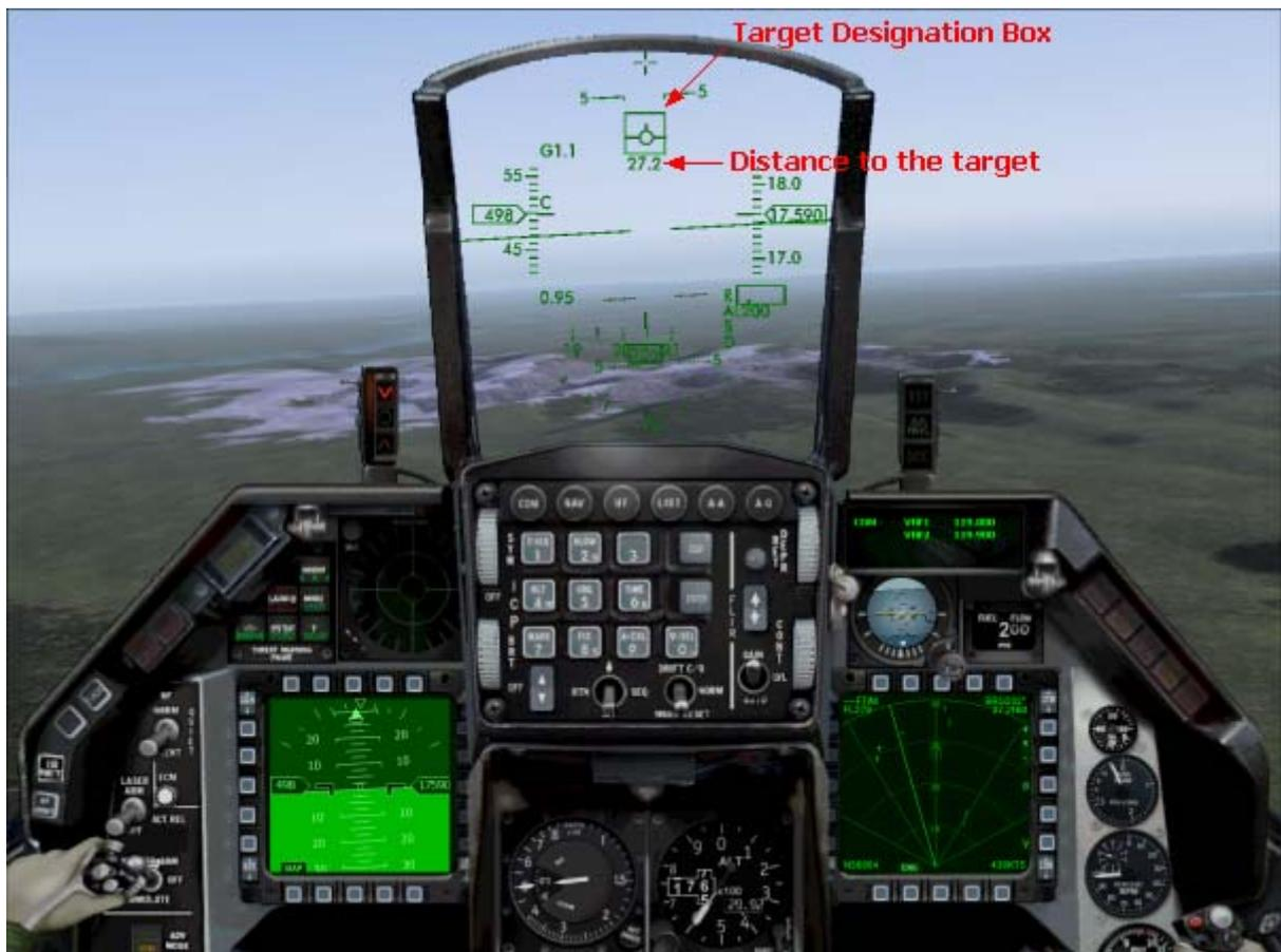
The target is at 27.2 NM, beyond visual range. The flight path vector is aligned with the target designation box to fly directly to the target.
