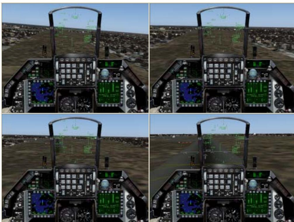
This landing sequence shows the aircraft is flying in the direction of the runway even if the nose is not heading to the runway. This is easily managed with the HUD flight path vector. The landing is not perfect because the flight path vector is not in the correct incidence range. The approach descent is too flat and the speed is too high, but this is safe when the wind is blowing.
