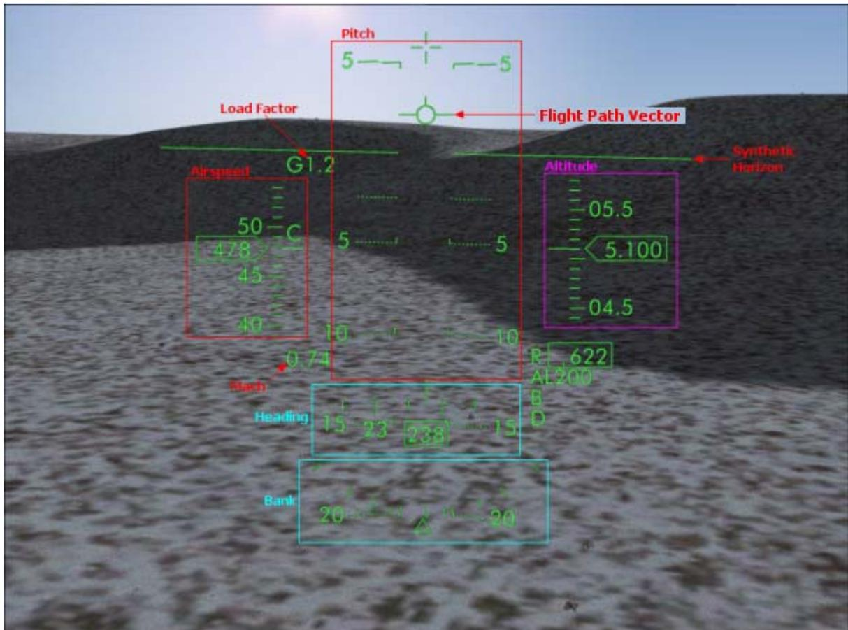
All the necessary flight information is displayed on the HUD so that you can fly the aircraft while looking outside:
