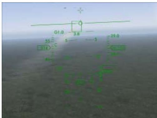
At 3.8 NM, the target is hardly visible (the contrails are visible), the designation box shows the direction.
