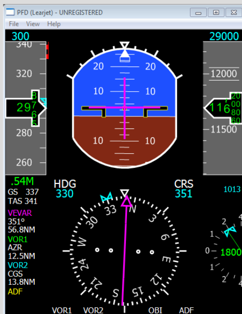
Primary Flight Display (PFD) running as a stand-alone application
