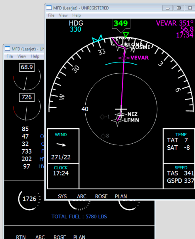
Multi-Function Display (MFD) displays navigation or engine information, depending on the display mode
